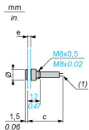
(1) Tags for Faston connectors or soldered connections
