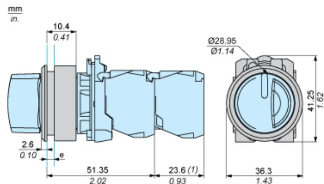
e : Clamping thickness : 1 to 3.5 mm / 0.04 to 0.14 in.
